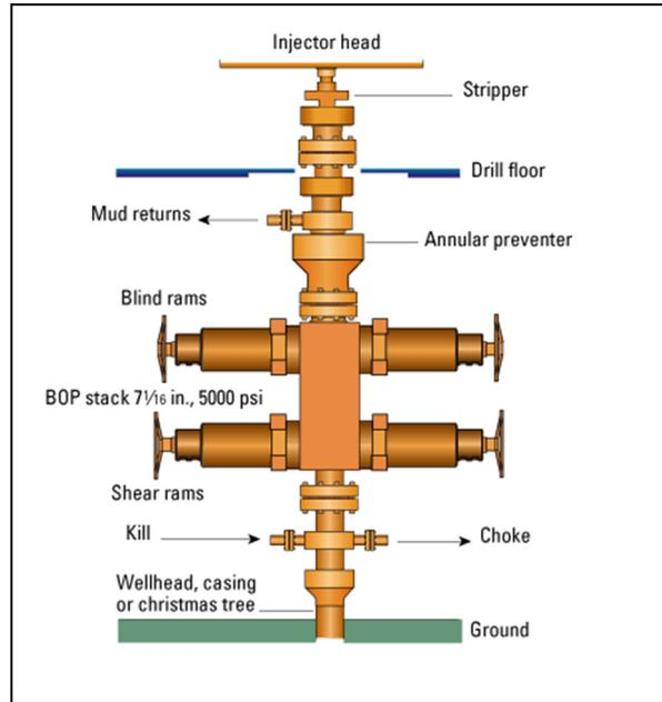
The stack consists of an annular ram, a blind ram, and a shear ram. The blind ram can close the well when an internal pipe (called the drill string) is not within the well. When the drill string is in the well, the shear ram can cut through the pipe and close the well.
