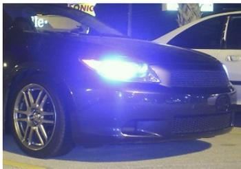
HID (High Intensity Discharge) lighting has proven its efficiency for the operator by providing more usable light. It has also been proven to have negative affects to blinding the oncoming driver due to the lighting intensity of the HID bulb. Another advantage of the HID is the useable hours of life are 2800 hours compared to the 450 – 1000 hours for halogen system.
